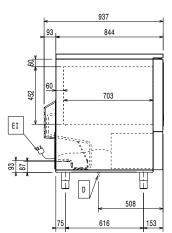
Drain Electrical inlet (power) ΕI Refrigerant Outlet
